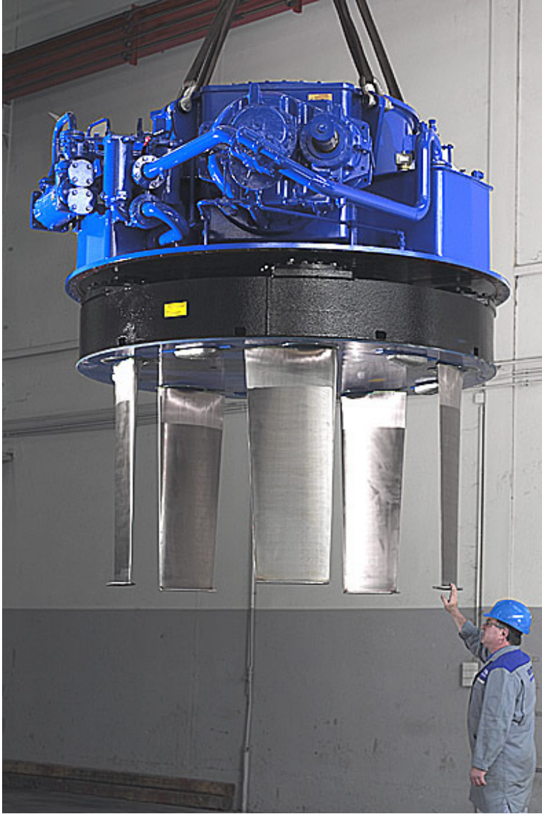
Figure 1 - A Voith Schneider propulsion unit of similar size to that fitted on W-Class ferries
