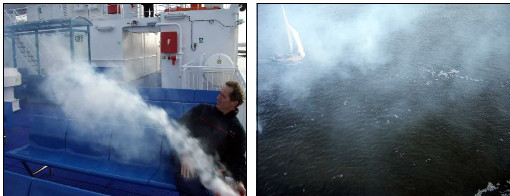
Figure 66: Flow Visualisation on W-class Sun Deck
