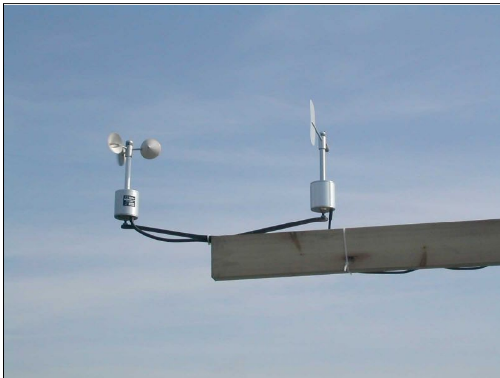
Figure A5.2: Anemometer and Arm on Pylewell Boom Navigation Post
