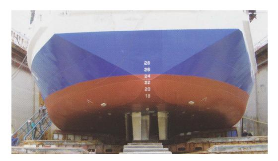
One of the much larger, more powerful and deeper set W Class VS thrusters. Only the bow thruster is used in the river as the wake from the other was deemed to be dangerous. The flow from it is forced between the hull and the river bed and banks.
