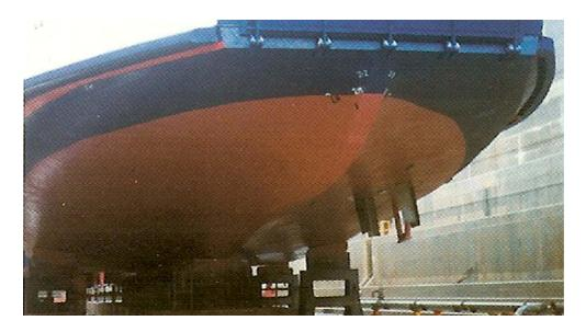
One of the smaller, shallower offset C Class VS thruster. Both thrusters were used in the river.
