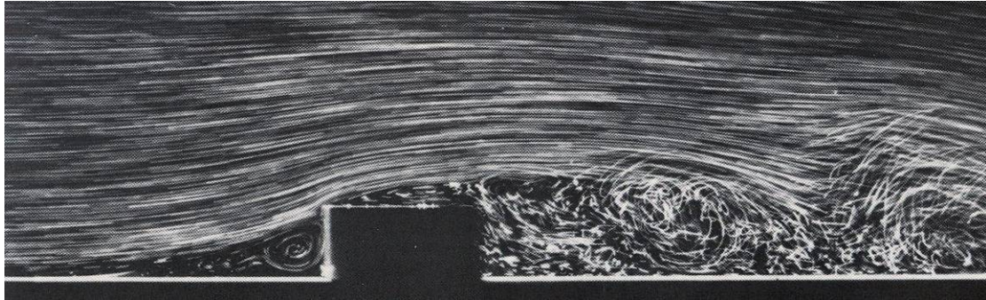
Figure 24: Flow Around a Bluff Body on a Surface. (from "An Album of Fluid Flow", The Parabolic Press, Stanford, California)
