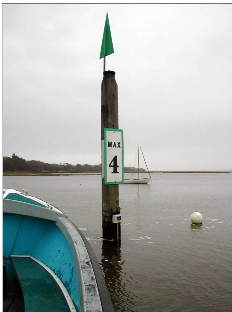
Figure A1: Water Level Probe Mounted on “Green” Post
